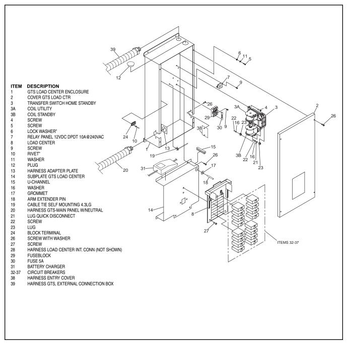
Figure 1. Exploded View of W/V-Type Transfer Switch
